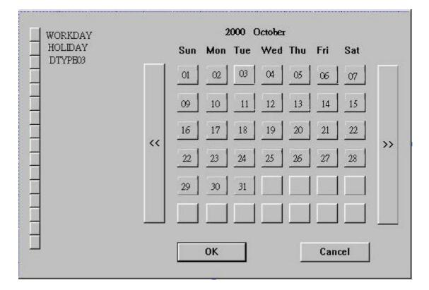
The active month is shown on the upper corner of the screen. The selectable Day Types are shown on the left corner of the screen. Please click on the Day Type button to select the active Day Type (the button will be on the DOWN position). Click on the Calendar Day button to change its Day Type to the active Day Type. Click on the << button to display the calendar days of previous month, >> button next month to the active month.
